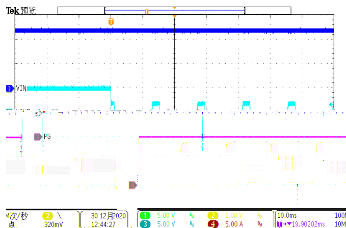
Figure 15. Over Current Protection(1A to hard short)
